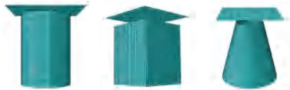
(a) 直四棱柱型柱吸能盒 (b) 圆柱型吸能盒 (c) 圆台型吸能盒
