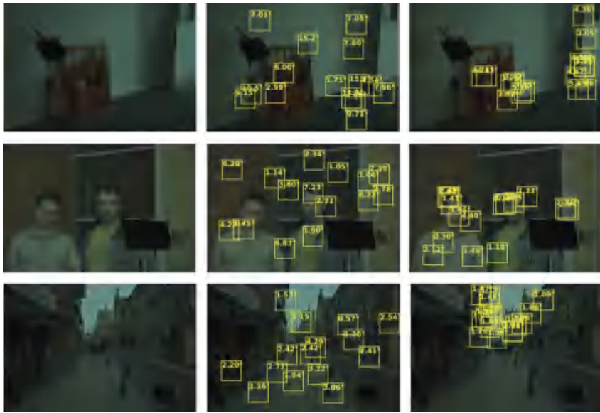
(a) 原始图像 (b) 随机采样方法的图像块分布 (c) 本文采样方法的图像块分布 (a) Original image (b) The patches distribution of random sampling method (c) The patches distribution of our sampling method
