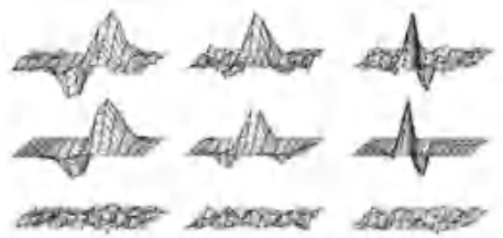
图 2 Gabor 小波滤波器和脊椎动物视觉皮层感受野响应的比较 Fig. 2 Comparison between Gabor wavelet filter and vertebrate visual cortex receptive field response
